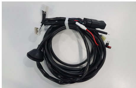
Central Locking Vehicle Loom - LV01 Code: C7B-LOOM-LV01
